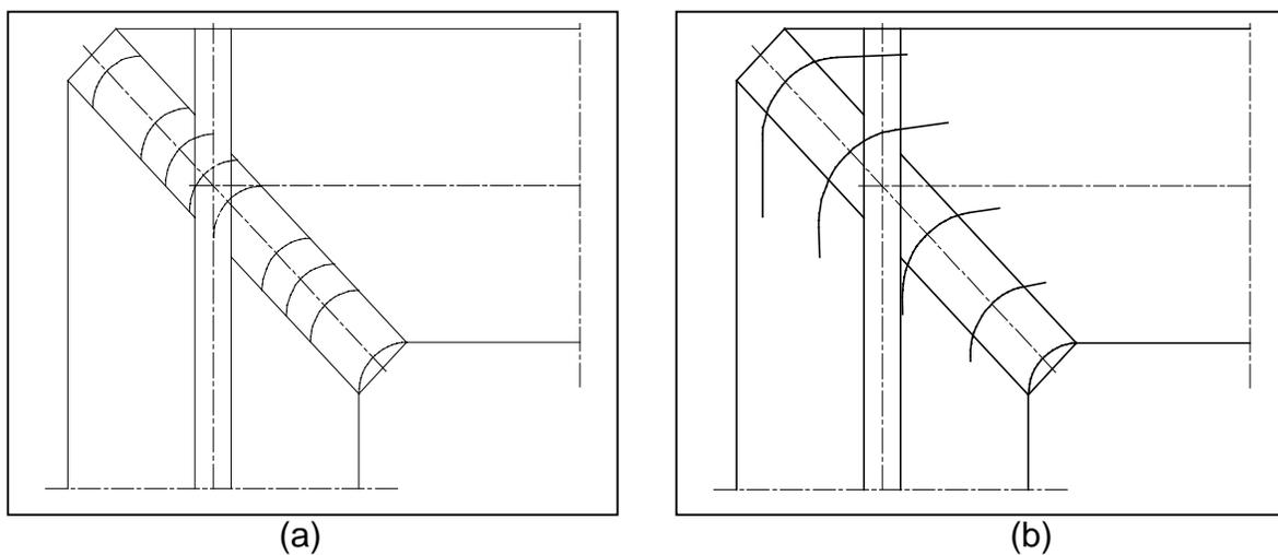
Figure 8: Comparison between existing (a) and new (b) elbow turning vanes
