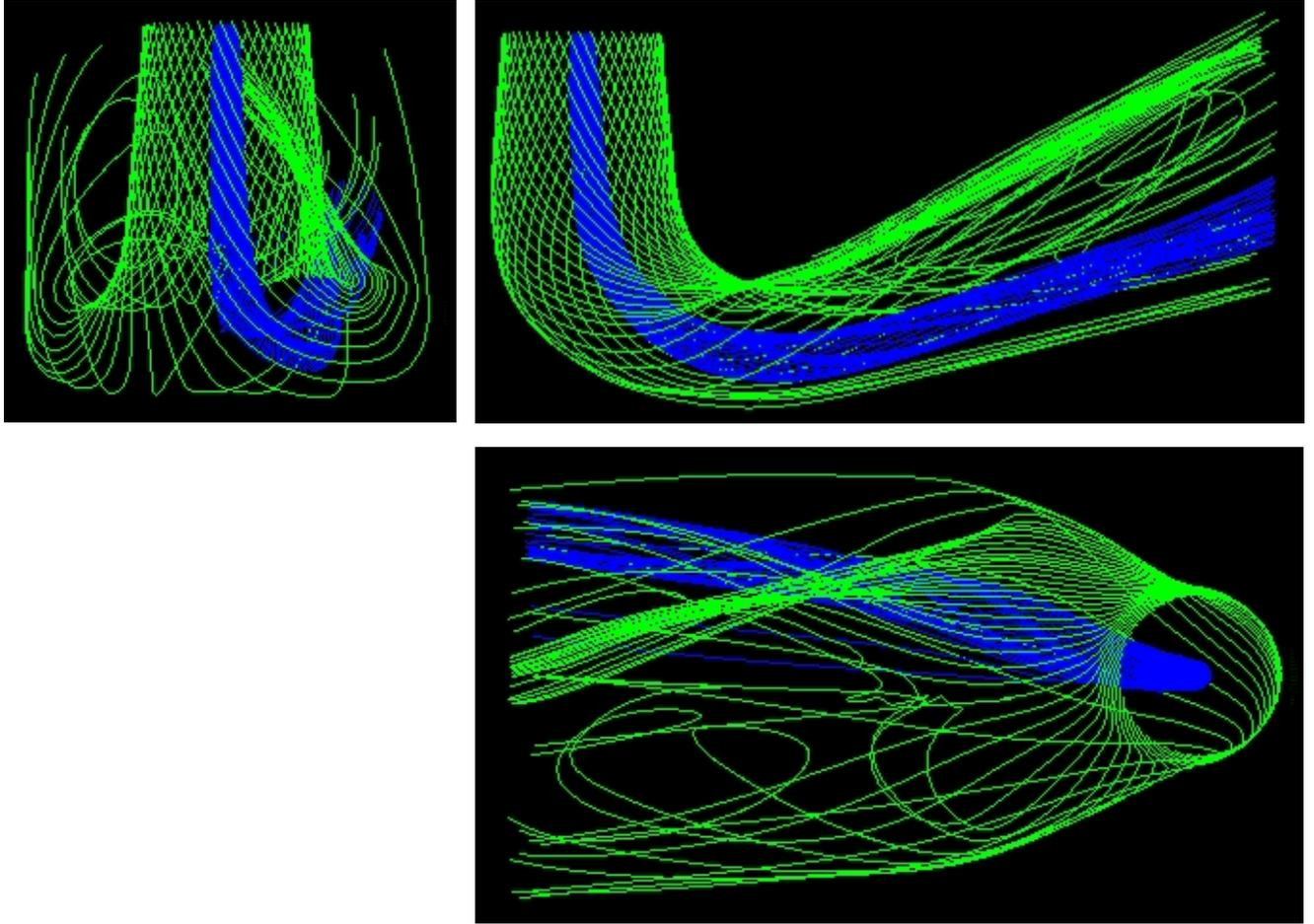
*Figure 6: Draft tube flow - CFD results for the existing draft tube with the new runner/distributor assembly*
