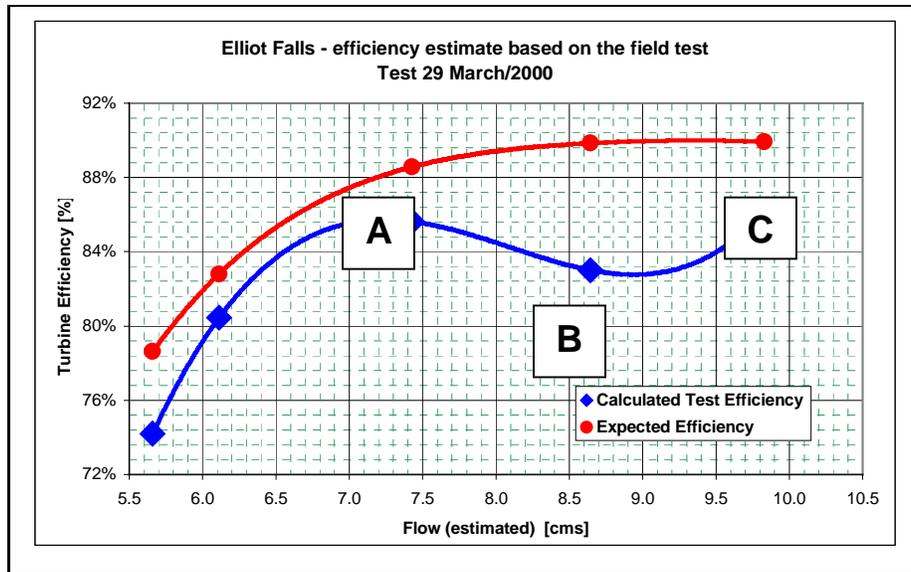
Figure 7: Estimated Efficiency of the runner/distributor/draft tube assembly
