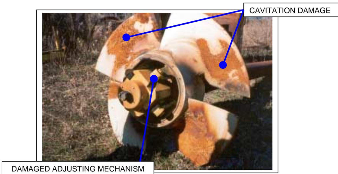
*Figure 1: Photograph of old blade and hub assembly showing cavitation damage and damaged adjusting mechanism (runner diameter is 5 feet).*
