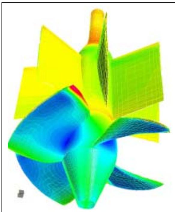
Figure 5: Static pressure distribution of the runner/distributor assembly
