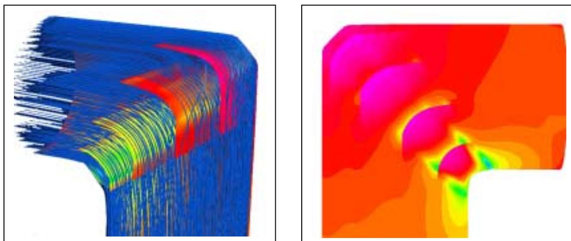
Figure 9: Results of the flow simulation for the new elbow turning vanes
