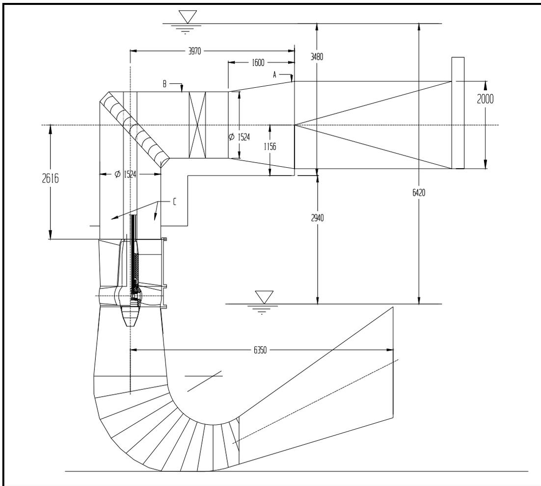
Figure 3: Elevation showing existing water passages and key dimensions
