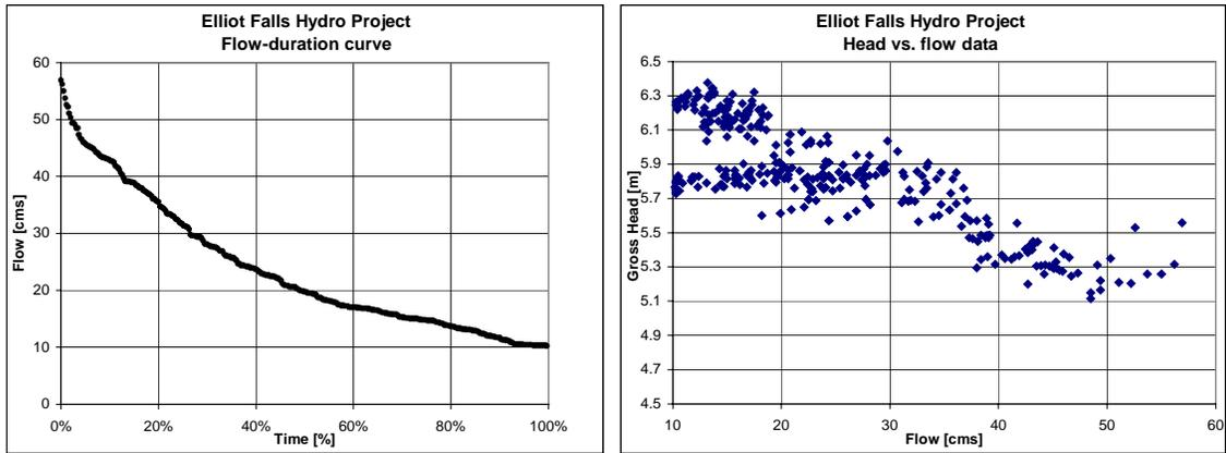
Figures 2 (a) and 2 (b): Data collected at the site over 5 years of operation.
