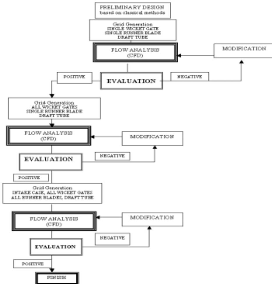
Figure 4: CFD design procedure adopted for the Elliott Falls runner/distributor assembly
