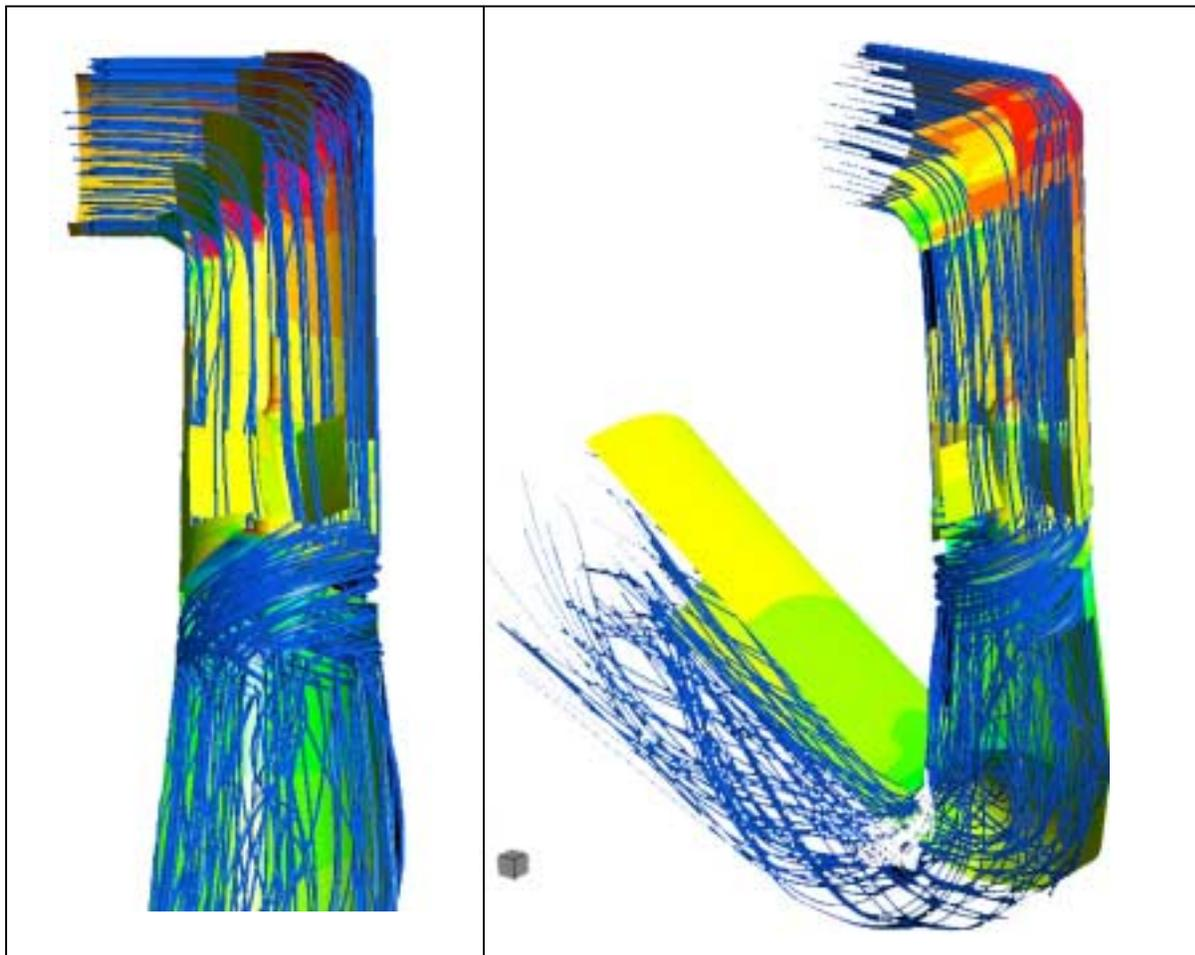
*Figure 10: Geometry of the entire turbine was used to evaluate the performance of the unit equipped with the new elbow turning vanes*
